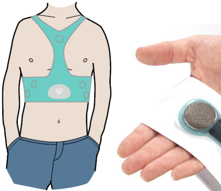
Figure 12. The 3-lead ECG vest and a textile electrode.
